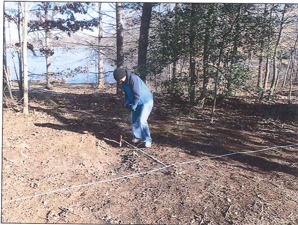
Photo 5: Caitlin Oshida Conducting the Penetrometer Survey Within the Study Area.
